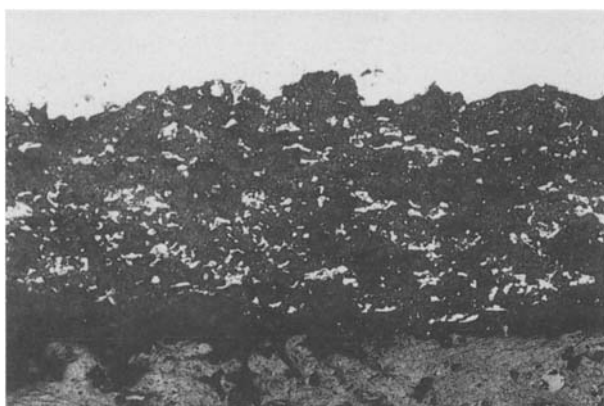
Figure 4 Metallographic cross-section of a coating with a Ni-20Cr bond coat and a ceramic overlayer of the sol-gel-derived YSZ. \times 100
